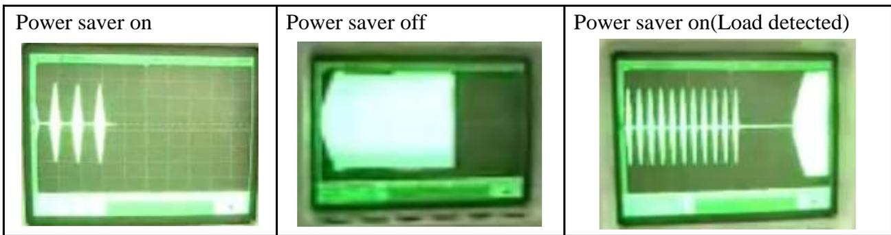
Note: The minimum power of a load to take inverter out of sleep mode (Power Saver On) is 50 Watts.
